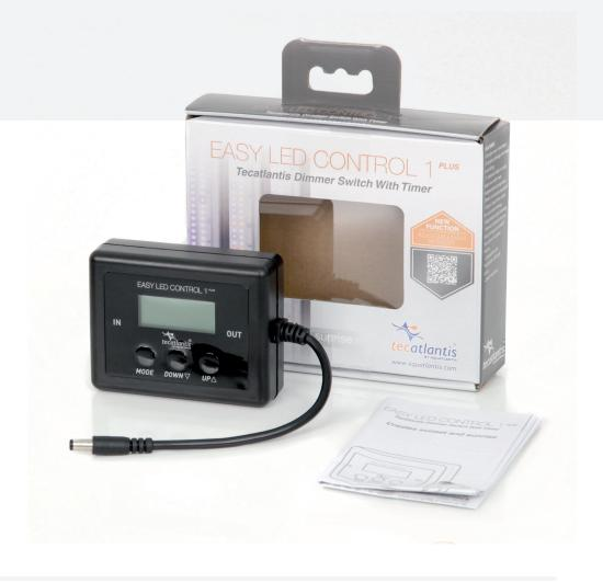
EASY LED CONTROL 1plus is a device which allows the EASY LED and EASY LED UNIVERSAL lighting to have more autonomy, allowing the operation to be programmed. The controller is connected to the power supply and programmed with the times for the lighting to switch on and off. At the scheduled time, the light unit will turn on and off gradually, simulating the effect of the sunrise and the sunset. It also includes a light intensity regulator (0% to 100%).
